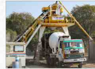
Machine : Batching Plant Company : Conmat Capacity : 21 CUM & 25 CUM/ HRS Number : 05 Nos.
