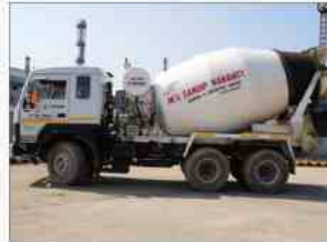
Machine : Transit Mixture Truck Company : Schwing Stetter & TATA Truck Capacity : 6 CUM Number : 07 Nos.
