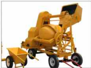
Machine : Concrete Mixer Company : Esquire / AMI Capacity : 0.3 Cum Number : 18 Nos.
