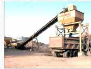
Machine : W.M.M Plant Company : Surelia Engg. Capacity : 180 M/ Hr Number : 01 Nos.
